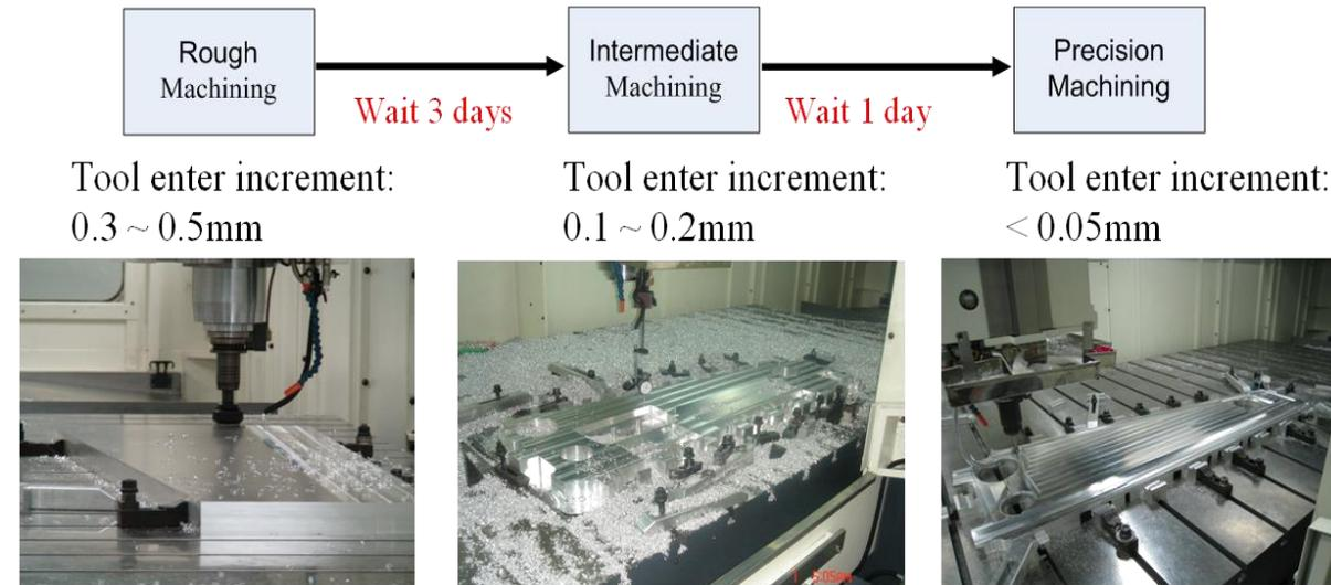
CNC Machining Processes (with 99.5% Ethanol as lubricant)
