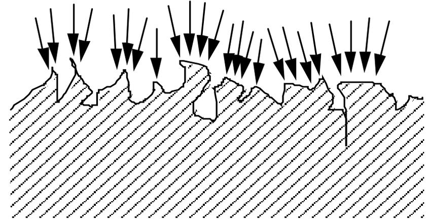
Resulting surface has reduced peaks, reduced surface area, and reduced outgassing
